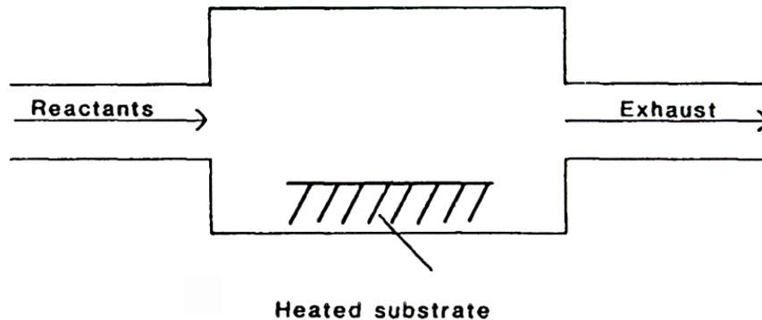
Fig. 3 Cold wall CVD reactor
