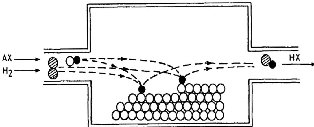
Fig. 1 Schematic of the chemical vapor deposition (CVD) process
