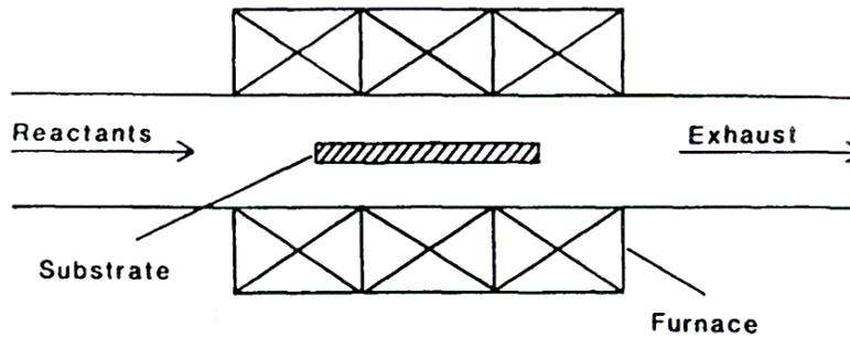
Fig. 2 Hot wall CVD reactor
