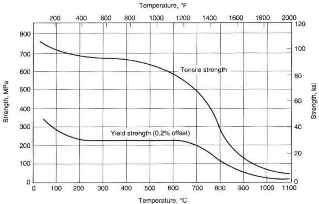
**Fig. 3 Effect of temperature on the tensile properties of an annealed 80Ni-20Cr resistance heating element alloy**
