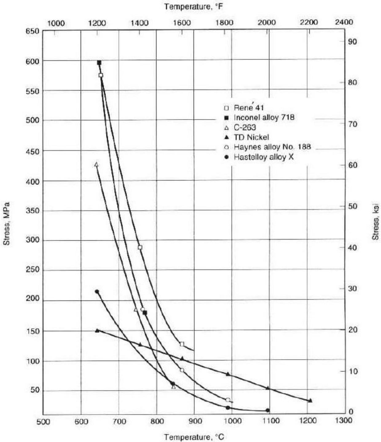
**Fig. 5** The 1000 h stress-rupture strength of TD Nickel and other heat resistant alloys
