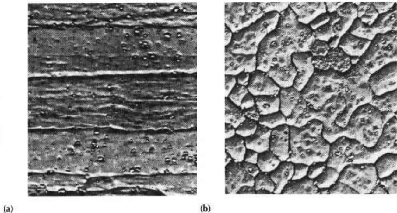
**Fig. 4 Replica electron micrograph of annealed TD Nickel sheet, showing grain structure and dispersion of  $\text{ThO}_2$ . (a) Longitudinal (rolling) direction. (b) Transverse section. Both at 7000X**
