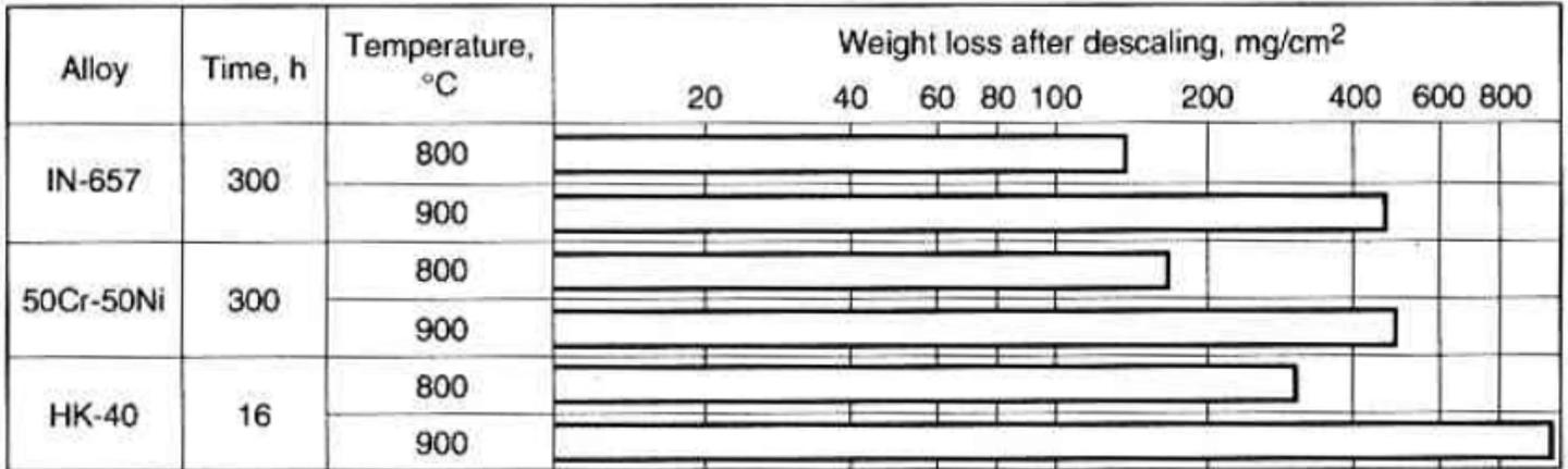
**Fig. 2 comparison of fuel oil ash corrosion resistance for nickel-chromium alloys and HK-40 steel**
