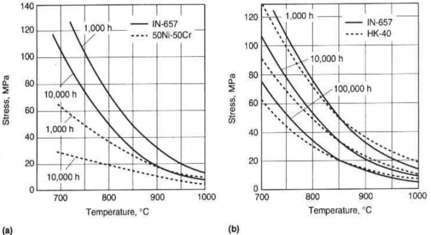
**Fig. 1 Stress rupture properties for Nickel Chromium and steel castings derived from Larson Miller Curve (a) IN-657 vs. 50Ni-50Cr. (b) IN-657 vs. HK-40**
